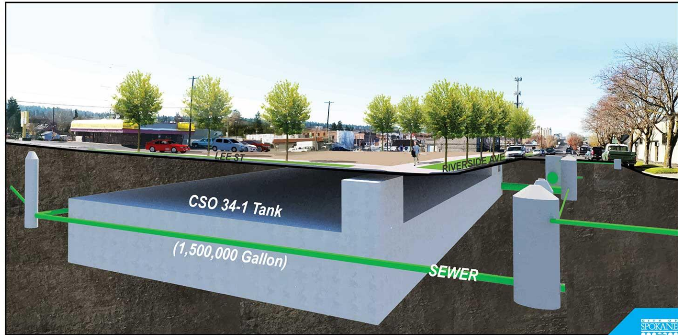
Combined Sewer Overflow Tank (CSO 34-1)
